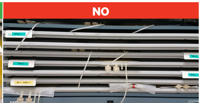
Image on the right shows containers and tubing hanging out of the shelves and too close to the sides.
